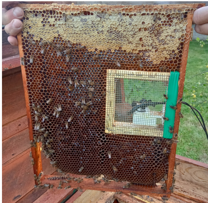
Figure 2. Photo of specialized protective enclosure mounted within a brood frame, protecting microphone from propolization and beeswax buildup. The setup is inserted into a lived-in frame as opposed to a new one in order to reduce the stress caused by foreign objects inside the hive. Photograph taken after measurements.
