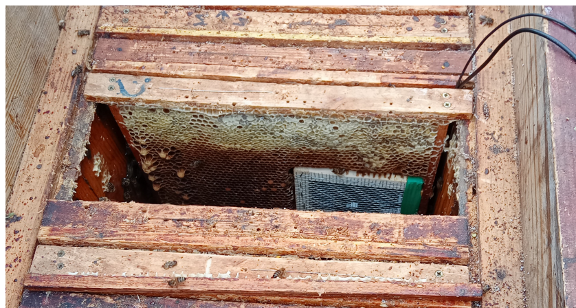
Figure 3. Internal microphone location after mounting the frame within the beehive. Photograph taken at the start of measurements; capped brood can be seen beside the setup.
