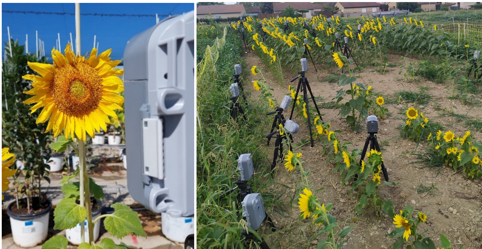
1164 Fig. 1. Left: Wingscapes camera positioned with the lens facing a sunflower head, on the Heliaphen platform. Right: Wingscapes cameras 1165 positioned on tripods in the field nursery of the INRAE site of Auzerville-Tolosane, France.
