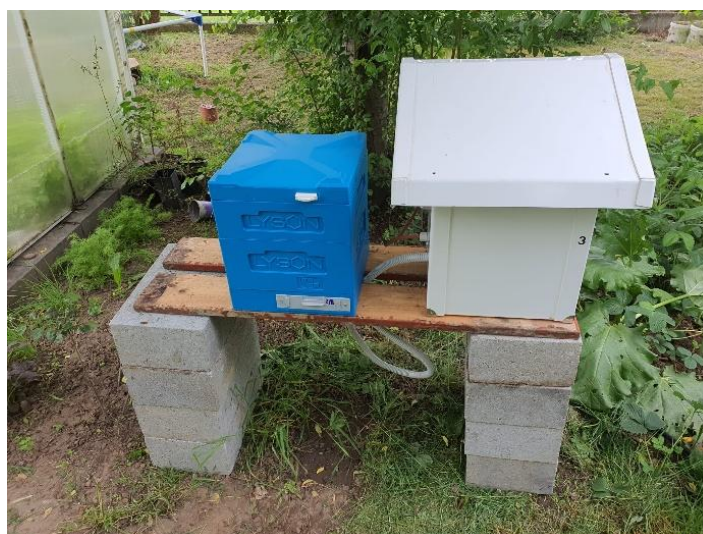
Fig. 5. An experimental stand for testing, in field conditions, the queen bee detection system. Left: twin-queen mating box fitted with two sensing modules, one module per queen. Right: Housing with data acquisition, processing, storage, and communication module and a gel lead-acid battery inside.
