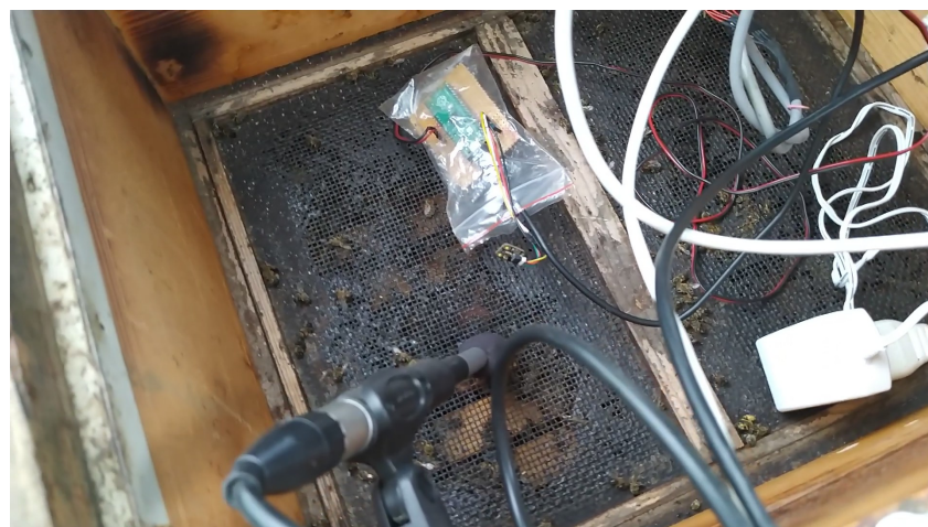
Figure 4. High-quality recording system and microphone-based embedded system in specially configured hive chamber.
