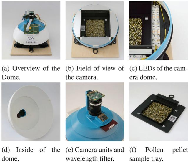
Figure 2: Detailed dome images: Detail images of (a) Pollen camera with mounted Raspberry Pi's, (b) Open pollen camera, scrim deflection of LEDs and pollen sample on sample carrier, (c) Detail view of the Illumination unit, (d) interior view of dome, (e) detail view camera unit. HQ camera in center of image with large black lens, tilted next to it, the IR camera and long-pass filter, (f) sample carrier with Petri dish.
