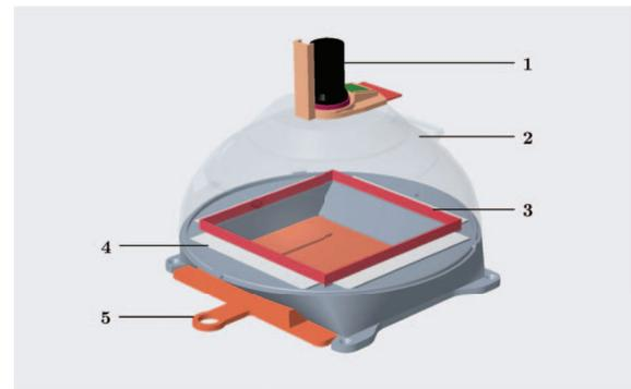
Figure 1: CAD model of the pollen camera dome (Camera Dome): The pollen camera consists of 1) camera unit including of Pi HQ camera (black), 2) dome, 3) lens hood, 4) illumination unit with four LED modules and 5) the sample carrier.
