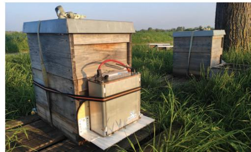
Figure 4: apic.ai Monitoring device attached to a hive at the Stutensee location. Bees are walking through the monitoring device into the hive. This hive has a bottom pollen trap and it is therefore not visible.
