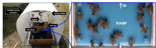
Figure 1. Video collection system and sample image that capture the honeybee behavior at the entrance of their colony.
