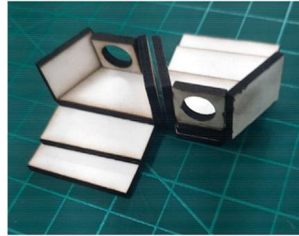
**Fig. 14.** Tentative design of beehive gate with step-wise ramp at the entry.
