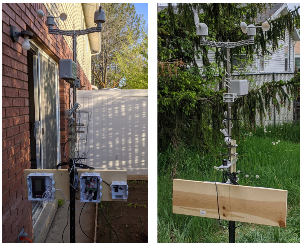
Figure 1. The left picture shows a weather station during a trial run in Logan in a small backyard next to a brick wall with a window; no data were collected at this site. The right picture shows the back side of the same station deployed at a private 6-hive apiary in Logan, where the weather and electromagnetic radiation data were collected from May 16 to 1 September 2020 (see Figure 2).
