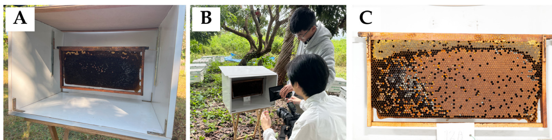
Figure 2. Experimental setups: (A) the Apis mellifera frame is placed on the holders inside the studio box, (B) the researcher made adjustments to the camera before image capture, and (C) an example of a frame from the image captured.
