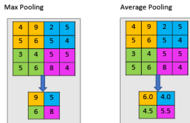
Figure 8. An illustration of the two pooling methods with a 2 \times 2 filter and a stride of 2 applied.
