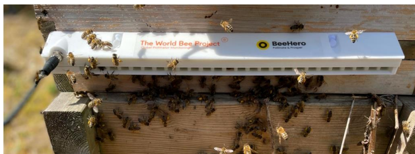
Fig. 8 Bee counting device [beehero.io]
