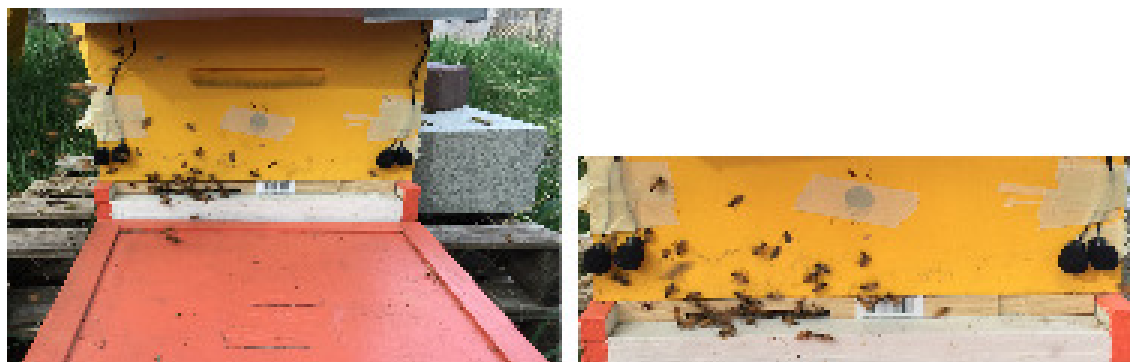
Figure 1. Four Neewer lapel microphones above Langstroth landing pad. The four microphones (two on each side of the pad) are placed approximately 10 cm above the Langstroth landing pad; four microphones are connected to the microphone hub inside the box with the BeePi hardware components placed on top of the hive; the microphones are not affected by rain or snow.
