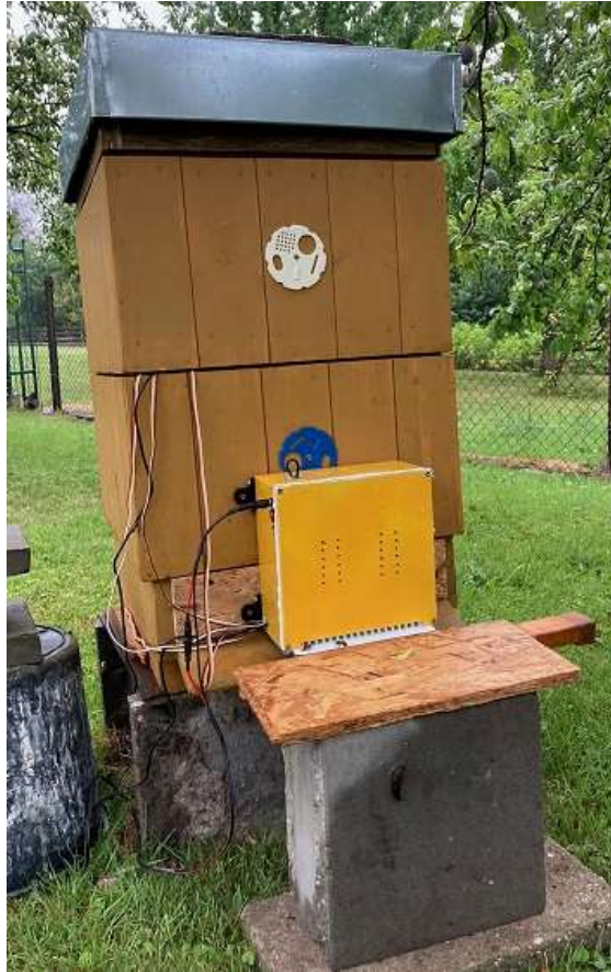
Figure 10 Bee health monitor in front of the hive
