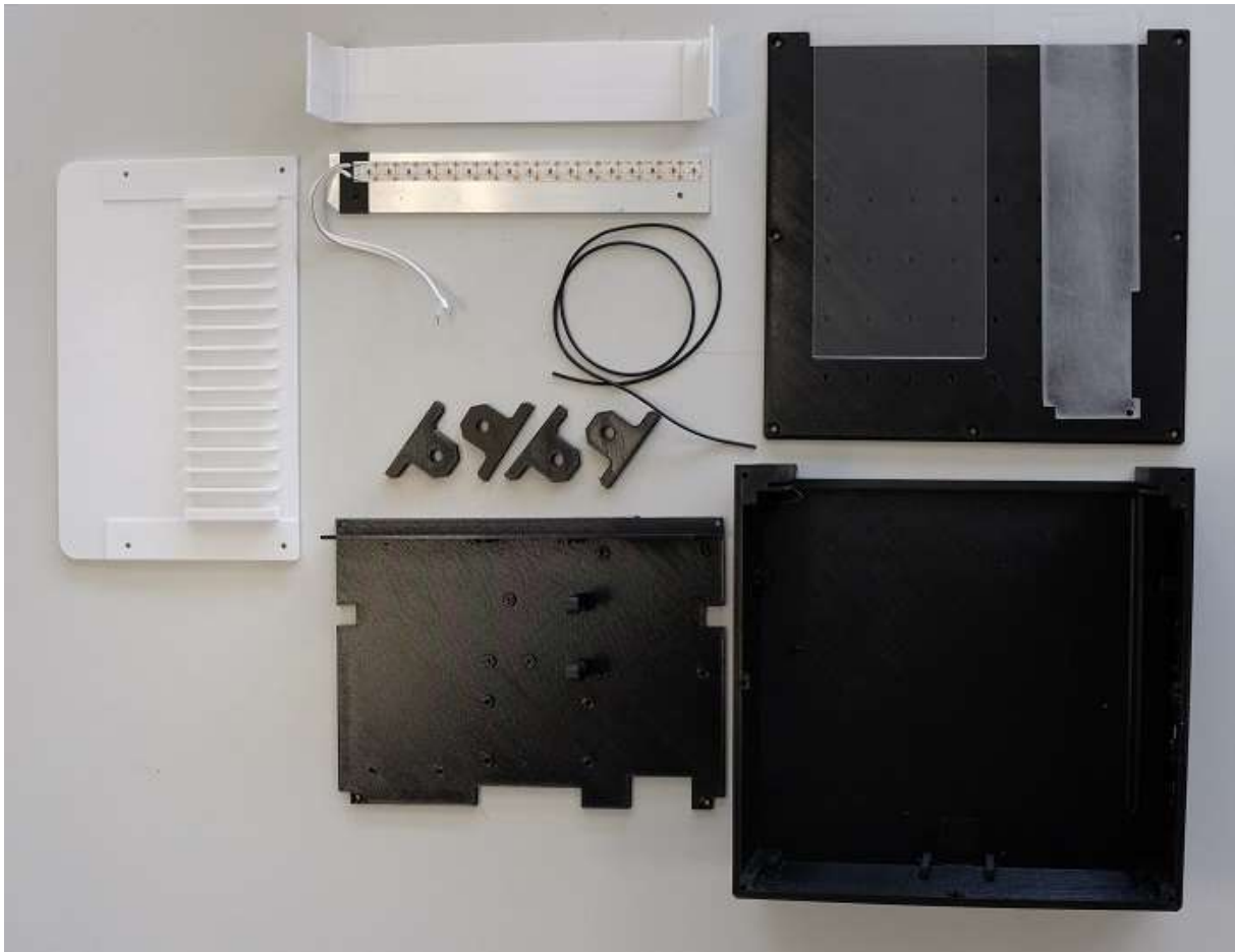
Figure 3 Printed 3D parts, laser cuts, LED plate and sealing gasket
